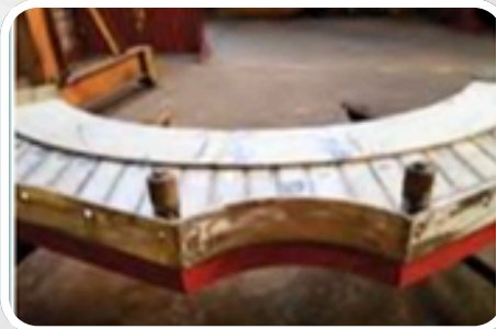
Water-cooled Center Smoke hood Section 2
