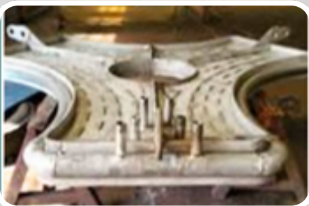
Water-cooled center Smoke hood section
